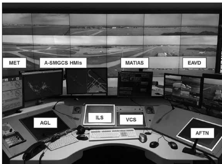
Figure 6. System of Remote Tower Controlling
